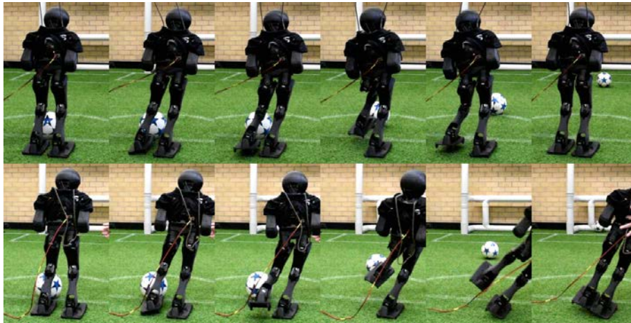
Fig. 3. Time-lapse of two of the kick scripts highlighted in Figure 2 – Ind_A (top) and Ind_B (bottom) – running on the real NUGus robot. In both cases, the distance travelled by the ball is very similar to the simulated results. However, only for solution Ind_A the robot still stands at the end, while Ind_B leads to the robot falling over – in the simulation, both scripts resulted in the robot standing at the end.
