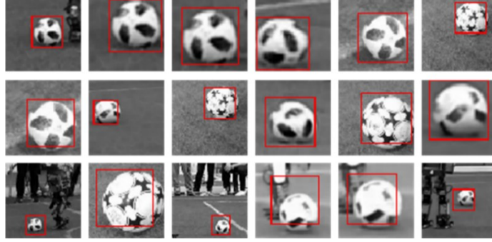
Fig. 5. The result of the ball detections with different IOU levels of P:0.9, P:0.75, and P:0.5 illustrated in the top, middle, and bottom row, respectively.
