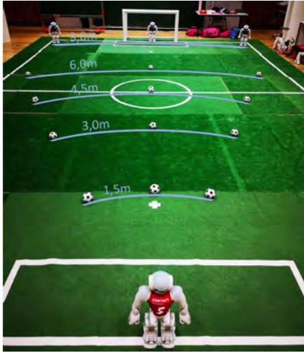
Fig. 5. Overview of the evaluation setup. We placed the robot that has to be detected on one the positions marked by balls after the other. The robot in the red jersey has to detect it.
