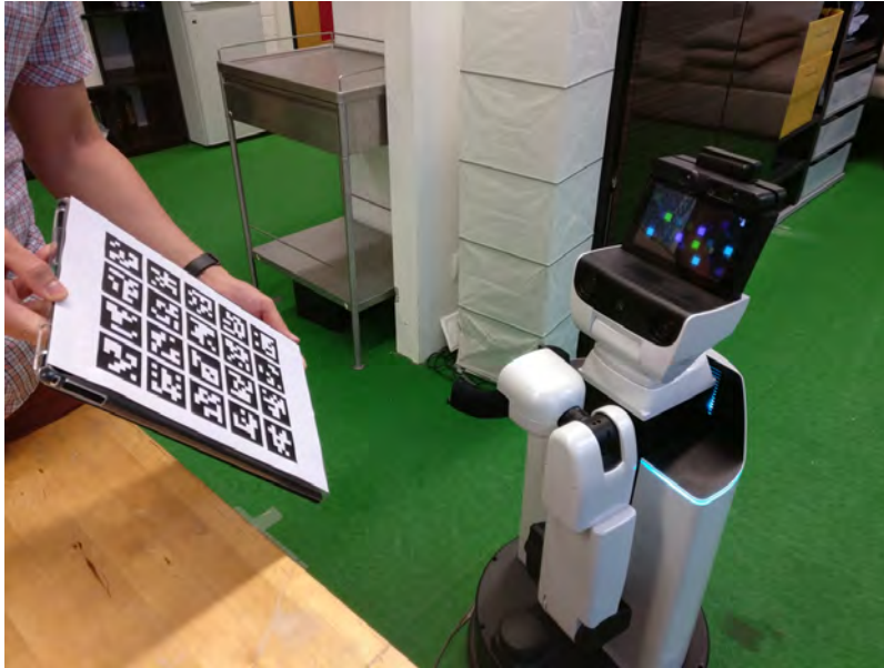
Fig. 2: DMP demonstration by observing an ArUco marker board
