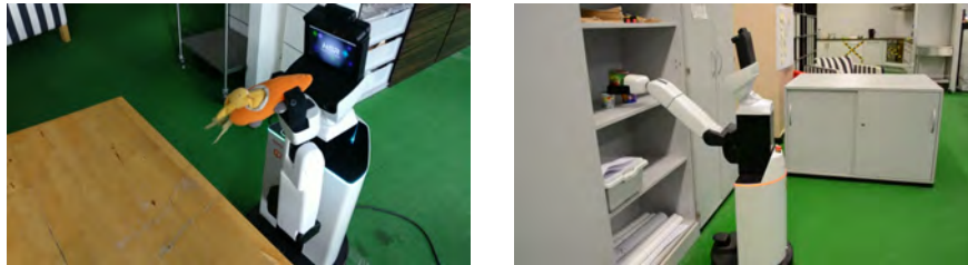
(a) A toy about to slip out of the gripper (b) The robot knocks down a yogurt cup
