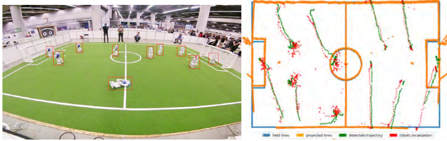
Fig. 7. Tracking of the robots on field conditions during the Ready phase. Left: final positions of the robots in the READY phase. Right: trajectories of the robots determined based on the video [green] in comparison to the communicated positions of the robots [red]. Projected line points are also shown in comparison to the model of the field. Note the goal posts being treated as lines.
