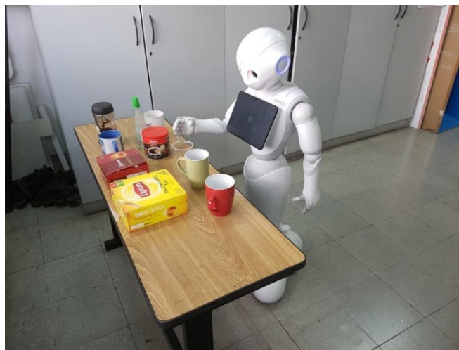
Fig. 1. Pepper robot detecting instances of domestic objects.
