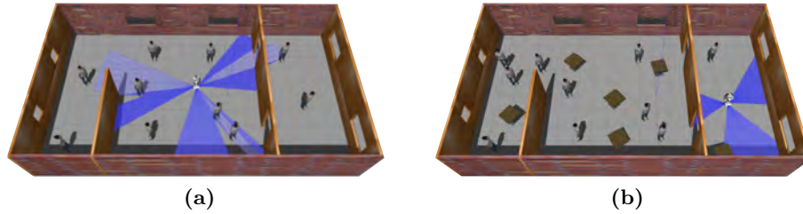
Fig. 4: Virtual environments constructed for training and validation in simulations. (a) Environment used for Experiments 1 and 2. Contains 10 simple obstacles (persons). (b) Environment used for Experiment 3. Contains 10 simple obstacles (persons) and 6 complex obstacles (tables).
