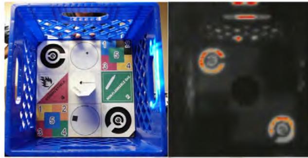
Fig. 7. The detection of thermal activity in a standard test crate (Courtesy RoboCup Rescue Technical Committee).
